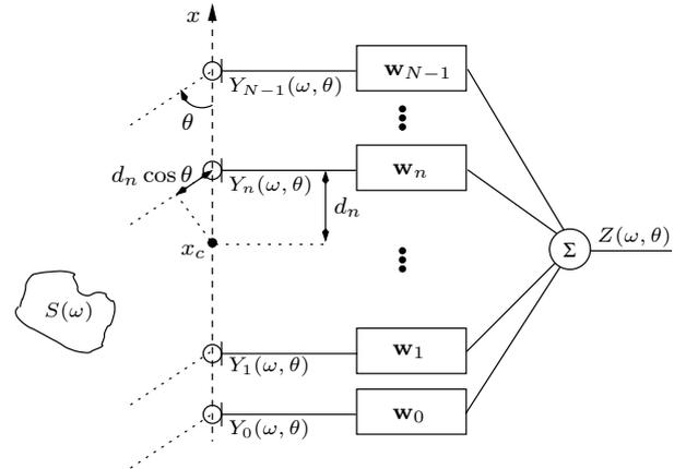
Fig. 1. Microphone array configuration (far-field assumption)
