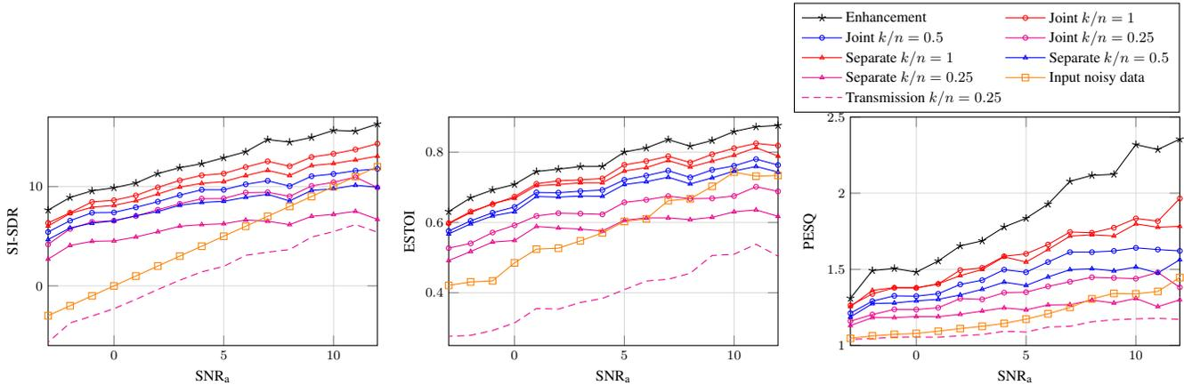
**Fig. 2:** Performance of the proposed joint enhancement and transmission methods for different bandwidths in terms of speech intelligibility (ESTOI), speech quality (PESQ), and reconstruction quality (SI-SDR) versus  $\text{SNR}_a$  of the speech signal against background noise. Curves with the same circle marker and triangle marker belong to joint and separate training systems, respectively, and curves with the same colour belong to the two systems with the same bandwidth.
