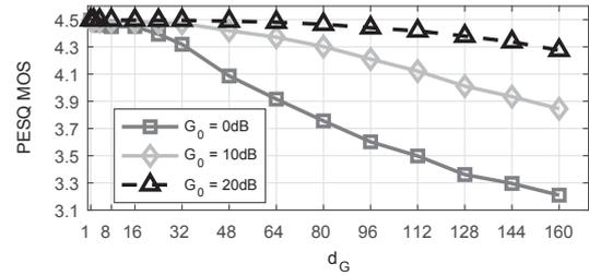
**Figure 7:** PESQ MOS values of the occluded ear signal at the ear drum  $t_{occ}[k]$  as a function of the forward path delay  $d_G$  for different forward path gains  $G_0$ .
