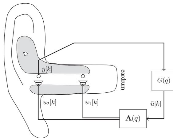
**Figure 1:** Schematic overview of considered single-microphone multi-loudspeaker custom hearing earpiece setup.
