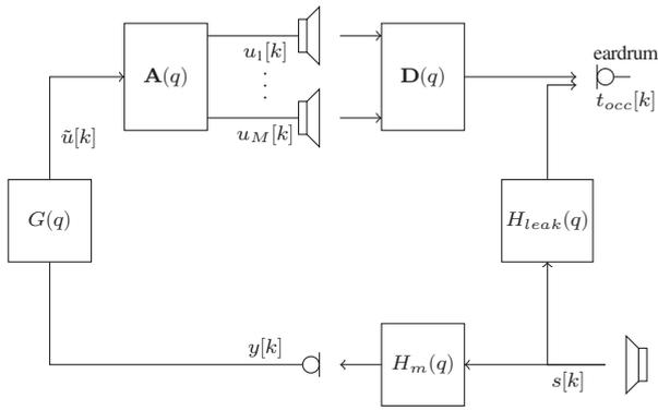
**Figure 2:** Generic single-microphone multi-loudspeaker hearing device setup considered in this work.
