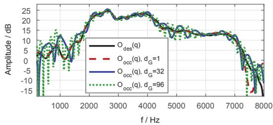
**Figure 5:** Amplitude responses of the system transfer functions for the occluded ear  $O_{occ}(q)$  and the processed open ear  $O_{des}(q)$  for different delays  $d_G$  of the forward path using a forward path gain  $G_0 = 0$  dB.
