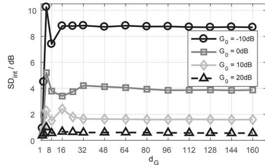
**Figure 6:** Speech intelligibility weighted signal distortion as a function of the forward path delay  $d_G$  for different forward path gains  $G_0$ .
