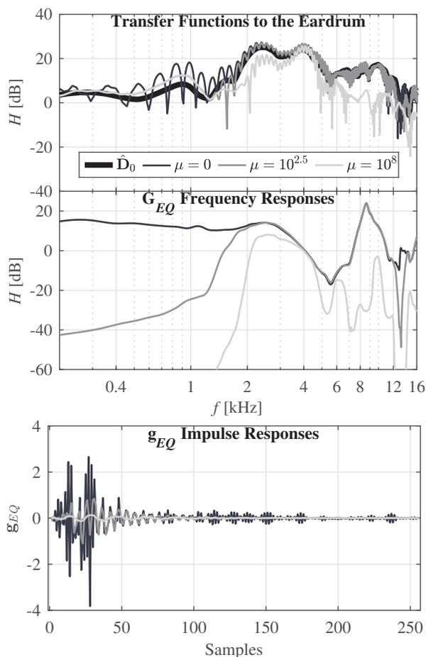
**Figure 4:** Top panel: Target and achieved aided transfer functions,  $g_{EQ}$  computed using Eq. (15) with different regularization parameters  $\mu$ , filter length of  $N_T = 256$  and  $D = D_{proc} + 24$ , i.e., and excess delay of 0.5 ms, as in Figure 3. Middle Panel: Frequency response of the equalization filters. Bottom Panel: Corresponding time-domain filter coefficients  $g_{EQ}$ .
