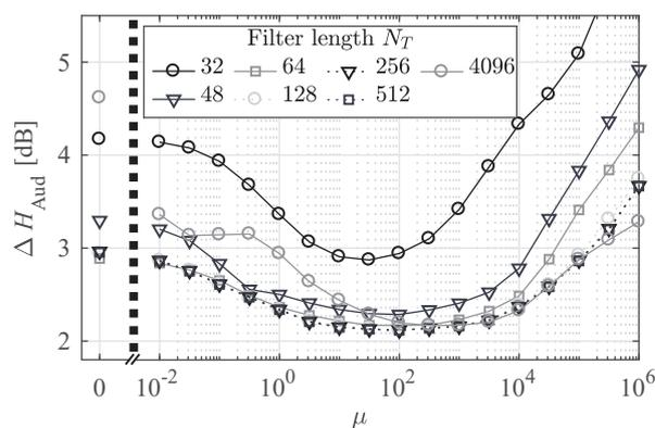
**Figure 5:** Auditory spectral distance between target and aided transfer functions with  $g_{EQ}$  computed using Eq. (15) depending on the regularization parameter  $\mu$ , with  $D$  set to the processing delay + 24 samples (= 0.5 ms)
