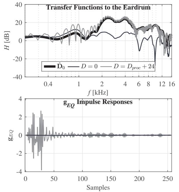
**Figure 3:** Top panel: Target and aided transfer functions,  $\mathbf{g}_{EQ}$  computed using Eq. (9) and Eq. (12), without ( $D = 0$ ) and with ( $D = D_{proc} + 24$ , i.e. 0.5 ms excess delay) including acausality management; filter length  $N_T = 256$ . Bottom panel: corresponding equalization filter coefficients  $\mathbf{g}_{EQ}$ .
