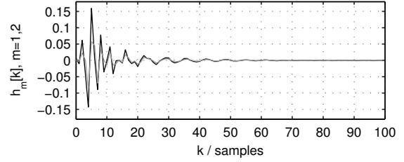
**Fig. 2.** Two measured feedback paths used in the experiment. The black line and gray line indicate  $h_1[k]$  and  $h_2[k]$ , respectively.
