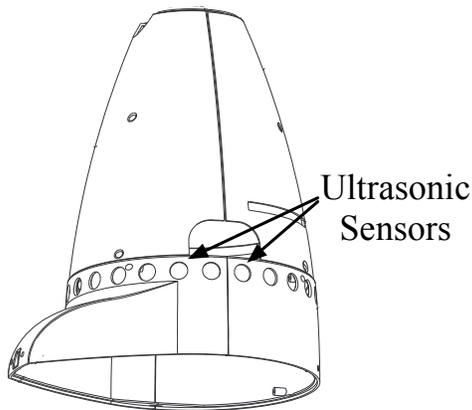
Figure 2: Lower part of the robot with ultrasonic sensors.
