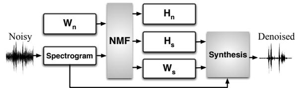
Figure 5: Overview of the NMF based denoising.
