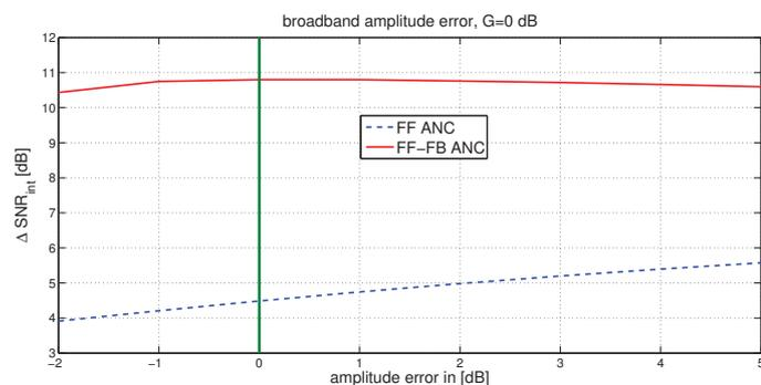
**Figure 3:** Speech intelligibility-weighted SNR improvement of the ANC-motivated algorithms depending on the broadband amplitude error in the secondary path estimation.
