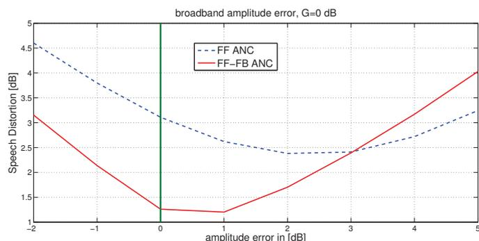
**Figure 4:** Speech intelligibility-weighted speech distortion of the ANC-motivated algorithms depending on the broadband amplitude error in the secondary path estimation.
