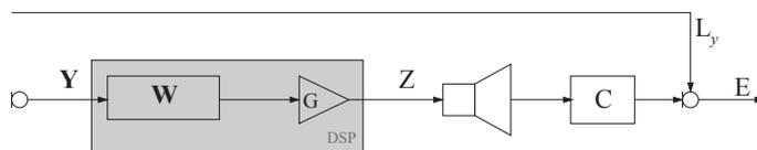
**Figure 1:** Hearing aid configuration with external microphones  $\mathbf{Y}$ , internal (error) microphone  $E$  and signal leakage  $L_y$ .
