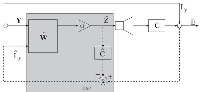
Figure 2: FF-FB ANC algorithm scheme
