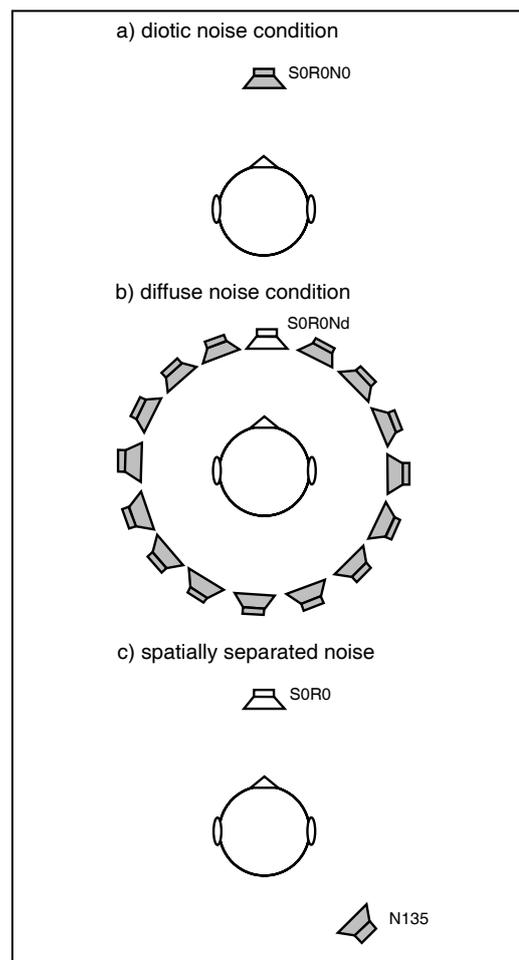
Figure 1. Sketch of the spatial arrangement of target speech, first reflection and noise sources.
