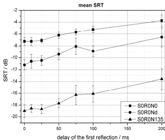
Figure 3. Mean SRTs and corresponding standard deviation for different delays of the first reflection in three noise conditions: diotic noise (squares), diffuse noise (circles) and spatially separated noise at  $135^\circ$  (triangles).
