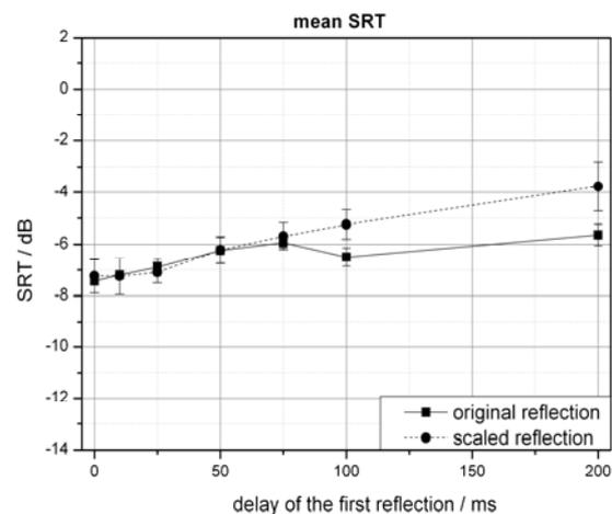
Figure 2. Mean SRTs and corresponding standard deviation for different delays of the first reflection with originally recorded amplitude (squares) and with scaled amplitude (circles) for 8 subjects.
