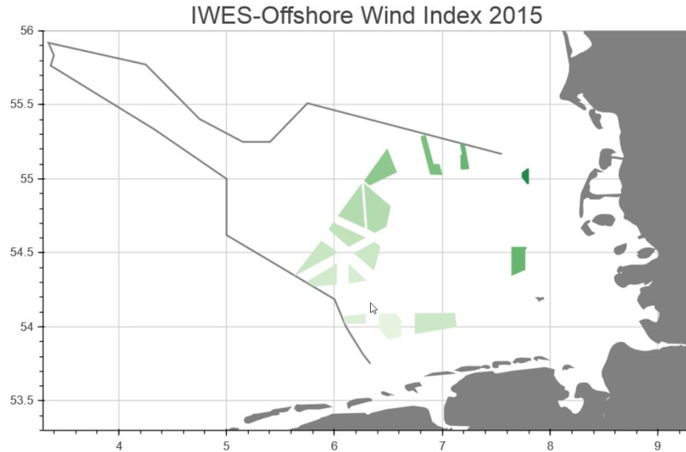
Relative local mesoscale wind and power analysis of time series calibrated by wind farm data
