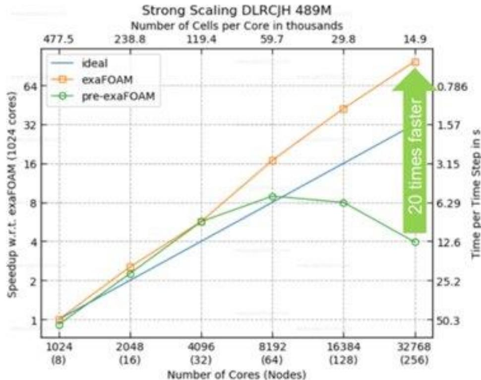
Older generation CPUs had an optimum of about 100k cells per core
