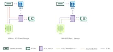
Source: https://developer.nvidia.com/blog/gpudirect-storage/ Examples for useable storage: local NVME drives, Lustre, BeeGFS, GPFS, WekaFS, VASTData, NetApp ONTAP, RDMA enabled NFS 28.09.2023 GPU Direct Storage: performance comparison
