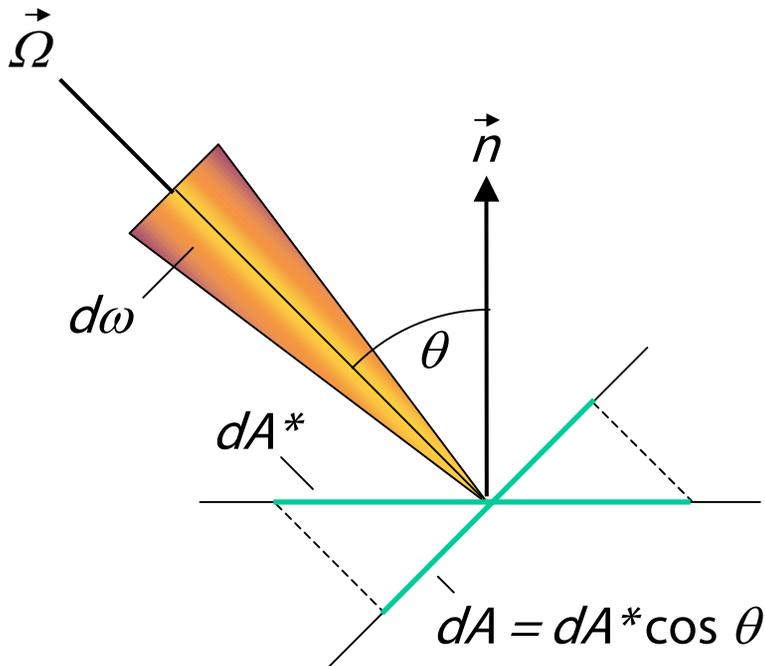
According to the cosine law, the radiance crossing a surface  $dA^*$ , whose normal  $n$  makes an angle  $\theta$  with the beam axis  $\Omega$ , is:
