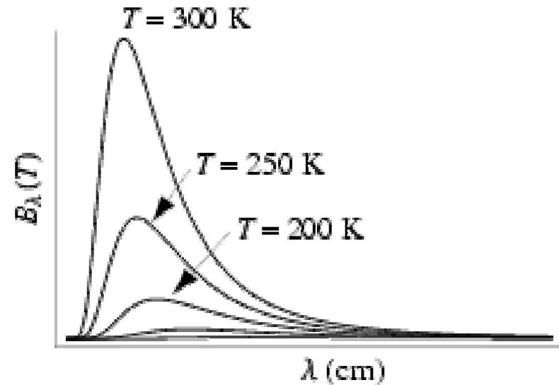
Intensity radiated by a blackbody as a function of frequency (left) or wavelength (right)
