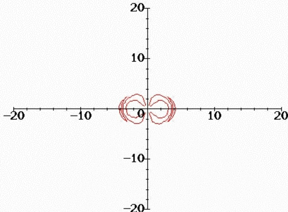
**Electric field lines due to an electric dipole oscillating vertically at the origin.**
