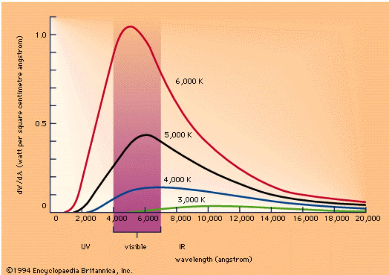
Electromagnetic energy  $dW$  emitted per unit area and per second into a wavelength interval,  $d\lambda = 1 \text{ \AA}$ , by a blackbody at various temperatures between 3000 and 6000 K as a function of wavelength.
