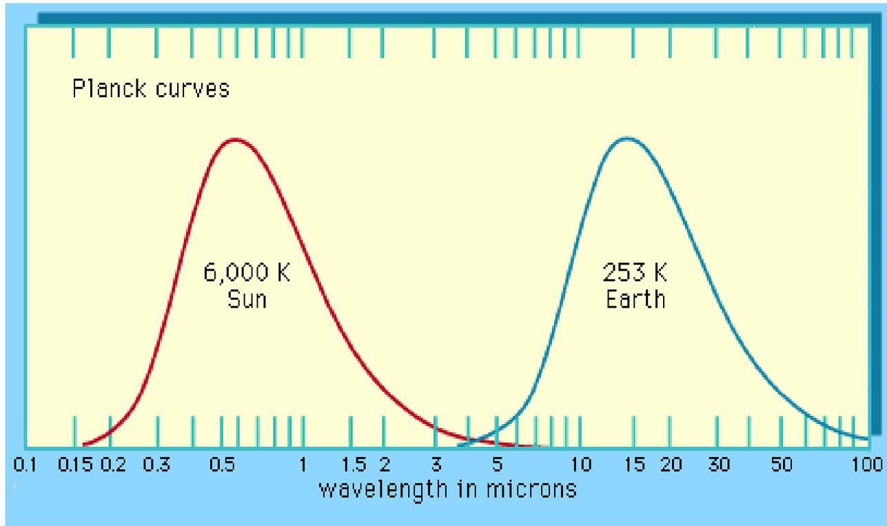
Spectrum of the Earth as viewed from space showing distinction between reflected sunlight and planetary radiation. The Earth is assumed to emit as a blackbody at an average temperature of 253 K.
