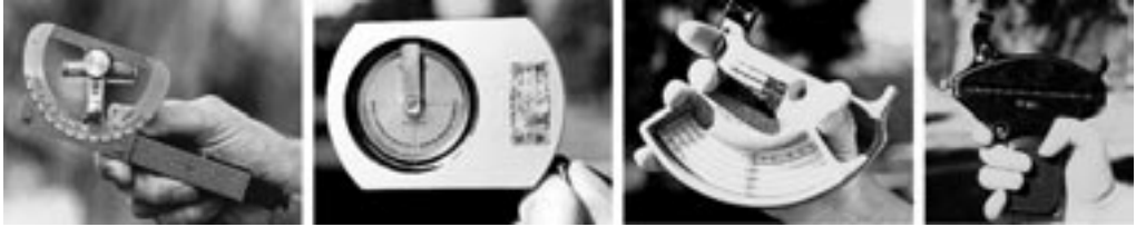
Figure 3.2. Instruments used for indirect tree height measurement, with from left to right the Abney level, Suunto, Blume Leiss, and Haga (Brack and Wood 1997).
