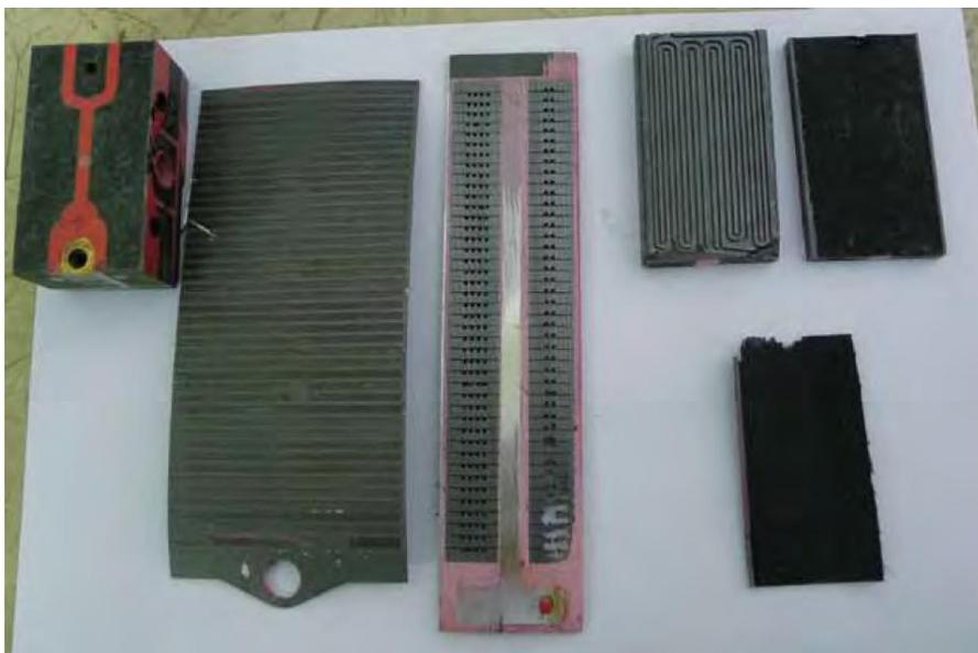
From top left: End adapter, contact plate, connecting element, unit of MEA and bipolar plate (shown from both sides), separated CCM
