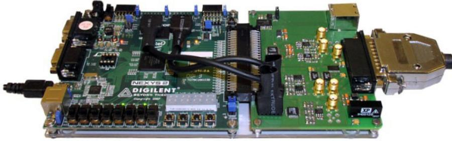
Figure 3.35: Picture of the developed scan generator.
