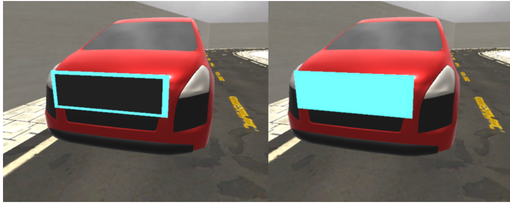
Figure 4.3: Visualization of the AV with an eHMI. Left: eHMI is off, the vehicle is cruising. Right: eHMI is on, vehicle will yield for the participant. Conventional vehicles did not have any light cues. Participants were introduced to different vehicle types in the game before the experiment.
